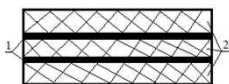
Fig. 2. Diagram of a cross section of the frozen fish block. 1 - aluminum spacer, 2 - layer of fish
