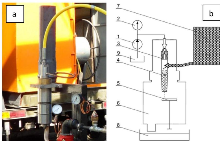
Fig. 1. Experimental setup for coal comminution efficiency research: a) general view, b) work schema: 1 – high pressure pump, 2 – manometer, 3 – water nozzle, 4 – comminuting and homogenizing nozzle, 5 – comminuting target plate, 6 – comminution chamber, 7 – feed container, 8 – product container, 9 – water tank.
