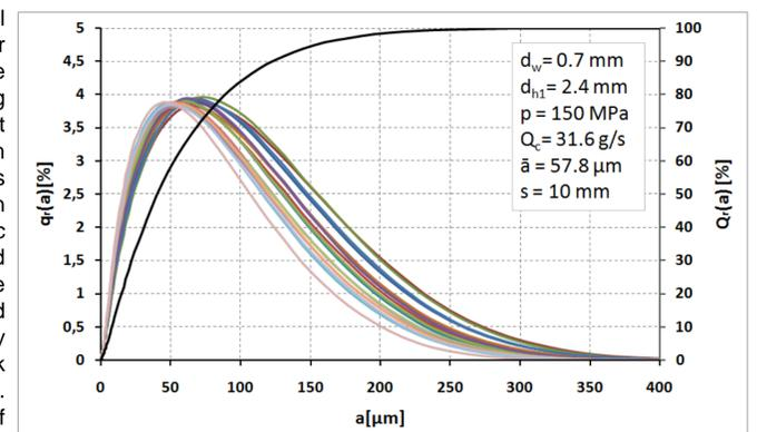
Fig. 2. Distributions of hard coal particles fraction comminuted with water pressure of 150 MPa.
