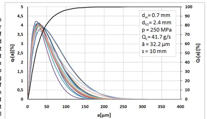
Fig. 3. Distributions of hard coal particles fraction comminuted with water pressure of 250 MPa
