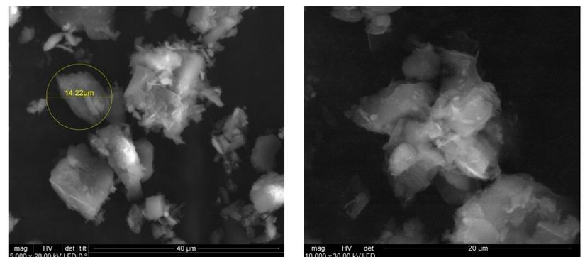
Fig. 4. SEM pictures of hard coal showing different stage of their specific surface development
