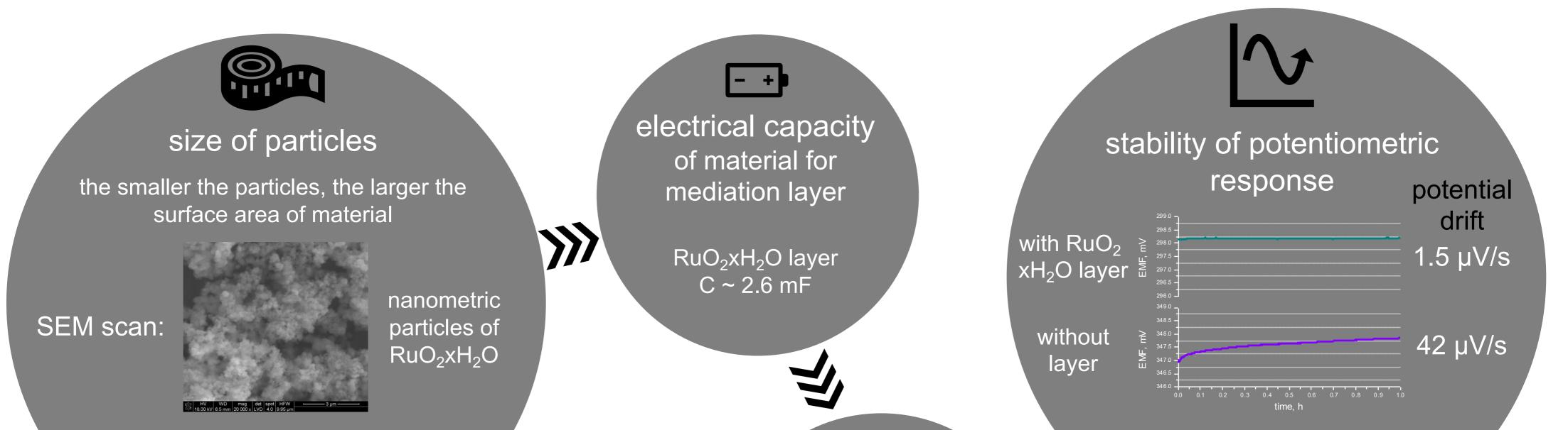
the larger the surface area, the greater the electrical capacity of material and, in consequence, of electrodes
