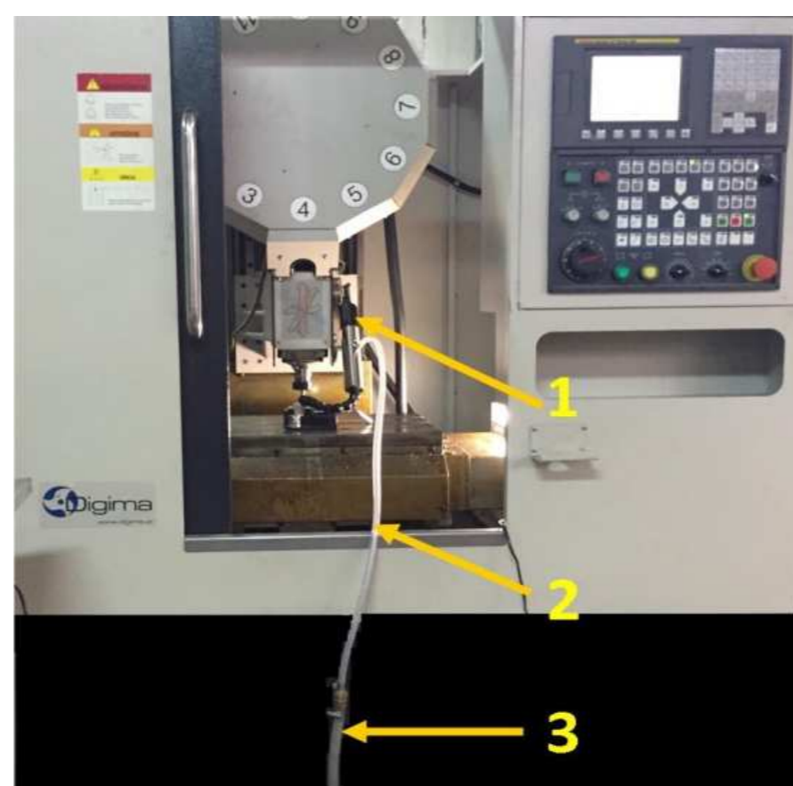
Fig. 3. Research station using Digima CNC numerically controlled machine tool. 1-cooling nozzle, 2-working CNC milling machine, 3-way compressed air supply [3]
