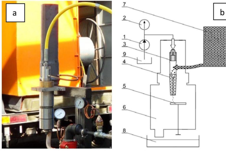
**Fig. 1.** Experimental setup for coal comminution efficiency research: a) general view, b) work schema: 1 – high pressure pump, 2 – manometer, 3 – water nozzle, 4 – comminuting and homogenizing nozzle, 5 – comminuting target plate, 6 – comminution chamber, 7 – feed container, 8 – product container, 9 – water tank.
